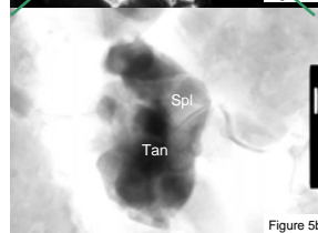
Fig. 5: a) Distribution of phases in a cavity between olivine clasts in Allende AF. The tiny, black grain in the middle of the micrograph is a compound grain of taenite and spinel as shown in the enlarged view (Fig 5b).
