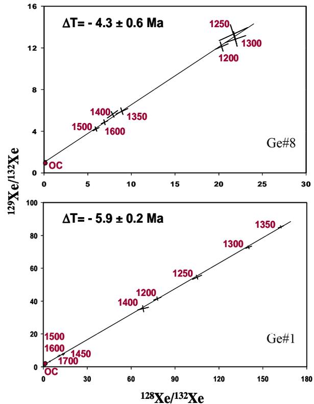
Fig 2. Three-isotope plots for Campo del Cielo silicates. Ages are shown relative to Shallowater ( $4562.3 \pm 0.3$  Ma [8]). OC stands for the Ordinary Chondrites component, numbers represent extraction temperatures.
