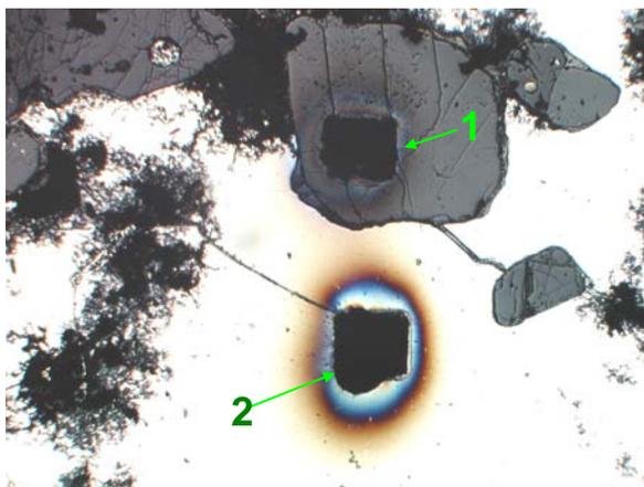
Fig. 1. Excavated 300×300 µm areas of Campo del Cielo iron. 1 – silicate (cpx inclusion ge#1, 2 – metal. Rust lace is visible on the left.
