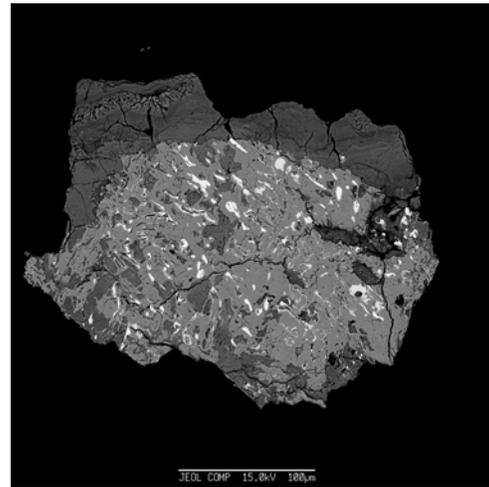
Fig.1. BSE image of particle NZ6-4-4,59 consisting of taenite and kamacite (white) embedded in Ni,Co-bearing Fe hydroxides (grey and light grey). A crust of Fe hydroxide without Ni covers the upper part of the particle.
