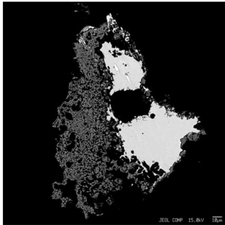
Fig.3. BSE image of particle NZ6-4-4,10. A porous aggregate of chromite (dark grey) on the left, Ni-Co-Cr metal (light grey, right) includes small precipitates of Cu-containing metal (white, upper center).
