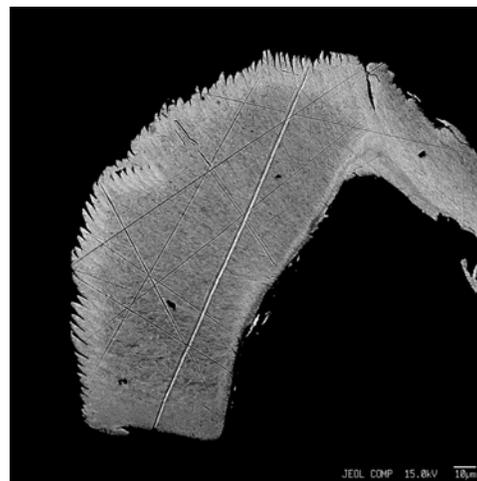
Fig.2. SEM image of all-metal particle NZ6-2-4,20. The lighter grey mantle contains more Ni and the inner part seems to consist of two phases.
