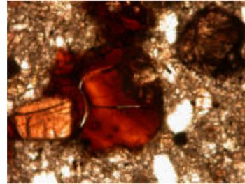
**Figure 2** Transmitted light image of glass fragment A4a. Note the intimate association of pyroxene (left) and glass.
