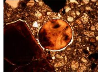
**Figure 1** Transmitted light image of glass fragment A1af (left) and glass sphere A1as. Note the schlieren outlining counter-flowing convection cells.
