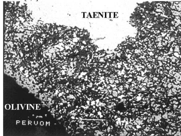
Fig. 4. BSE image of a taenite grain in Pervomaysky showing an outer rim. The rim consists of troilite (dark grey) with embedded fine low-Ni kamacite (light grey) and Ni-rich metal (white) grains. Scale bar = 10  $\mu$ m
