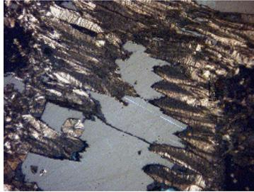
Figure 5: Detail of thin vein consisting of metal (gray) intergrown with feathery graphite growing from the crack wall. Optical picture, partly crossed polarizers, width ~680  $\mu\text{m}$ .
