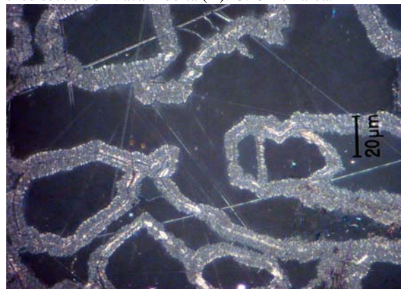
Figure 2: Graphite decorating grain boundaries between kamacite grains in Vaca Muerta K2. Note growth of graphite from grain boundary into metal. Optical image, partly crossed polarizers.
