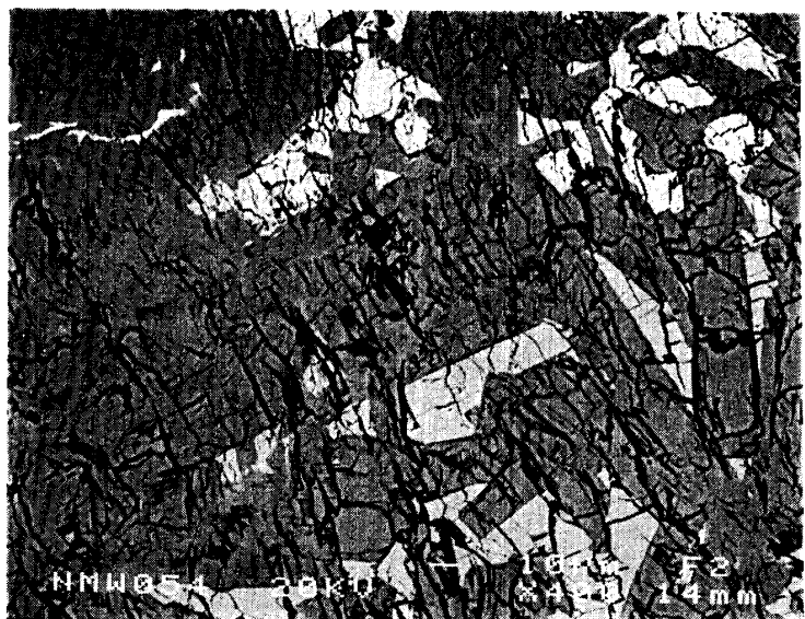
Fig. 13. BSE image of a meta-northositic gabbro clast from sample ,93 (part of clast WC2, see Table 5 for trace element data). The light gray ferromagnesian mineral in the upper part of the image is olivine, while the slightly darker mineral in the lower part is pyroxene.
