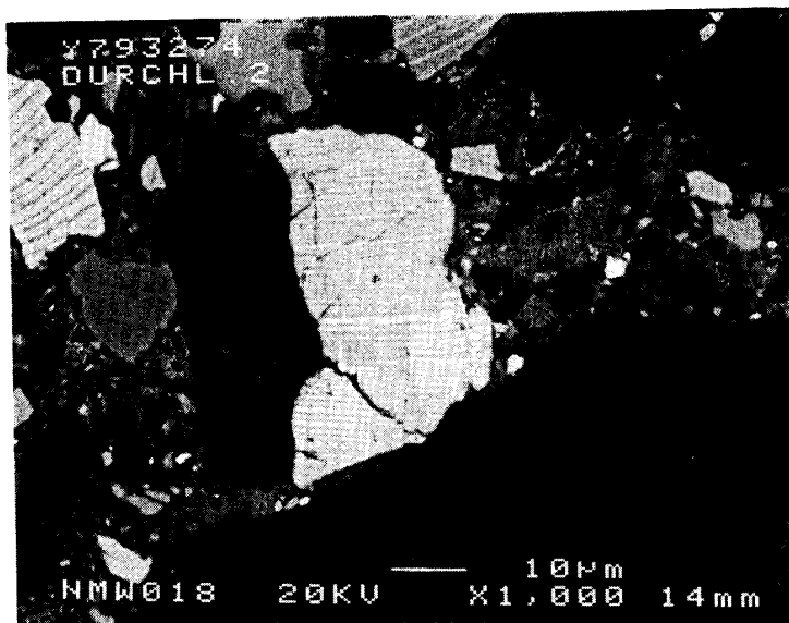
Fig. 6. BSE image of Fe-rich pyroxene with exsolution lamellae associated with silica (on the left side, dark gray) in matrix consisting of mineral fragments and devitrified glass. The large gray clast at the bottom of the image is plagioclase.
